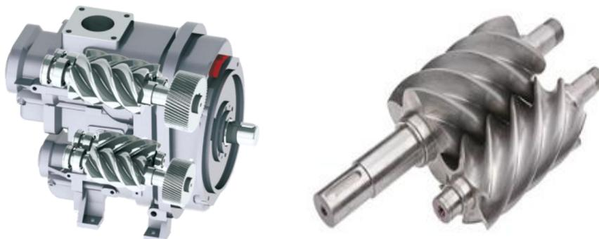
The rotor with bulging teeth outside of the pitch circle is called male rotor or male screw usually. The rotor with bulging teeth inside of the pitch circle is called female rotor or female screw. The male rotor is connected with the original electric
